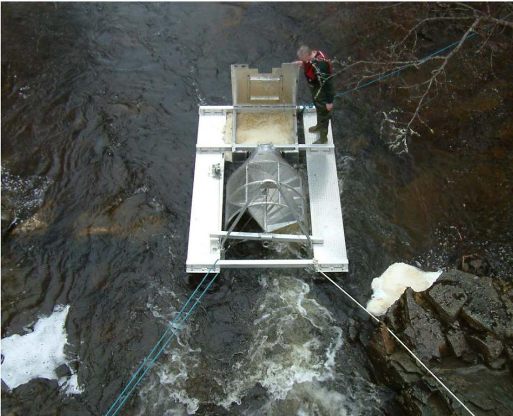
Figure 1b: Inspecting the rotary screw trap (4ft) for smolts, River Truim 2010.
