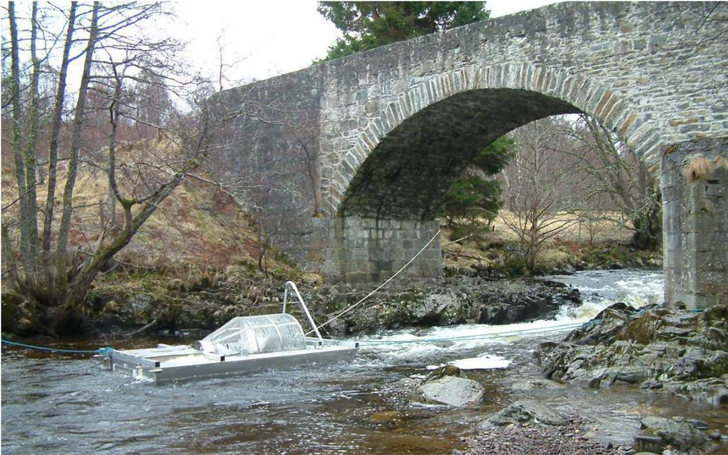
Figure 1a: Rotary screw trap (4ft) installed in the lower River Truim 2010.
