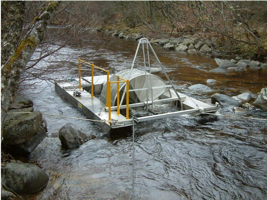
**Figure 1: Rotary screw trap (6ft) installed in the lower River Tromie March 2010.**
