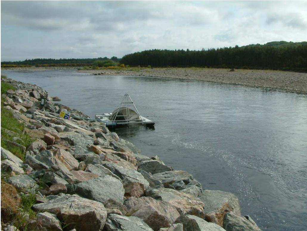
**Figure 1b: Rotary screw trap installed at Brae Beat 4, lower River Spey, 2006-08.**
