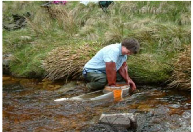
Janey Keay (Marine Scotland) collects invertebrates using a HESS sampler. The HESS sampler has a drum of known area which is placed on the river bed. The substrate is then agitated within the drum and the dislodged invertebrates are washed into the downstream net. (Photo: R. Laughton)
