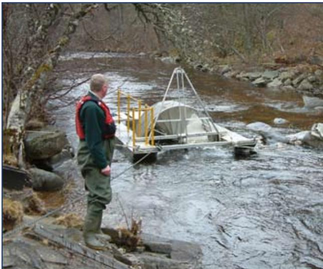
The 6ft Rotary Screw Trap installed on the River Tromie.
