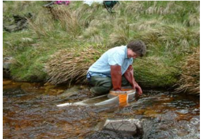
Janey Keay (Marine Scotland) collects invertebrates using a HESS sampler. The HESS sampler has a drum of known area which is placed on the river bed. The substrate is then agitated within the drum and the dislodged invertebrates are washed into the downstream net. (Photo: R. Laughton)
