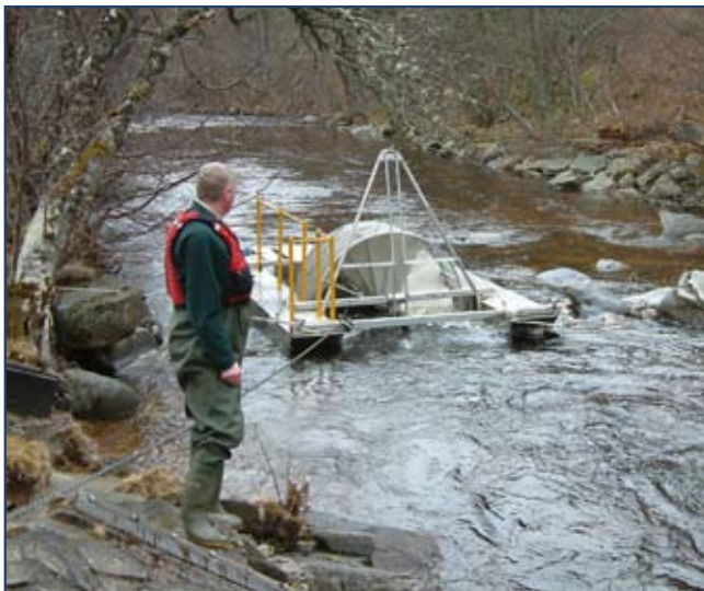
The 6ft Rotary Screw Trap installed on the River Tromie. (Photo R. Laughton)
